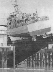
Out of its depth? *HMAS Gawler* in November 1997 in a position no ship want to find itself in. The result of a tsumani? Nope. Winching accident.
